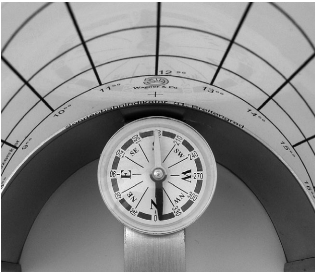
Figure 4: Use the compass to align the sun path indicator south, leveling it horizontally.
